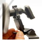
6 - Reattach the right side of the mount. Make sure the small lock washer is still on the lower screw and tighten untill the screw is fairly snug. Leave the top screw loose so the mount can slide along the mirror stem to the desired location.
