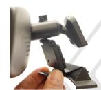
5 - Install this mount from the passenger side of the vehicle. Remove the right half of the mount by removing the two socket head cap screws. Be aware that there is a small lock washer on the lower screw. With the left half of the mount still attached, position the mount around the mirror stem as shown above.
